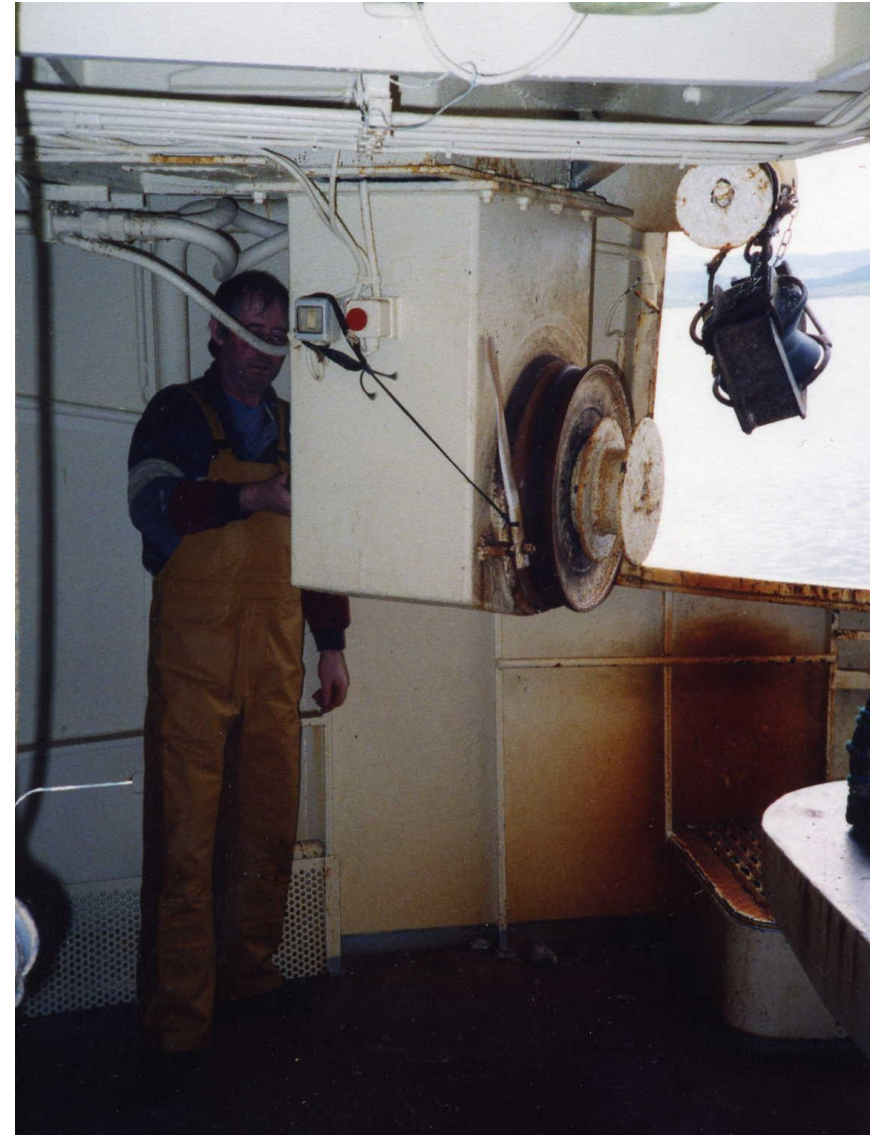
The overhead mounting arrangement allows the recovered main line to coil conveniently below the hauler, considerably simplifying the handling of the gear
