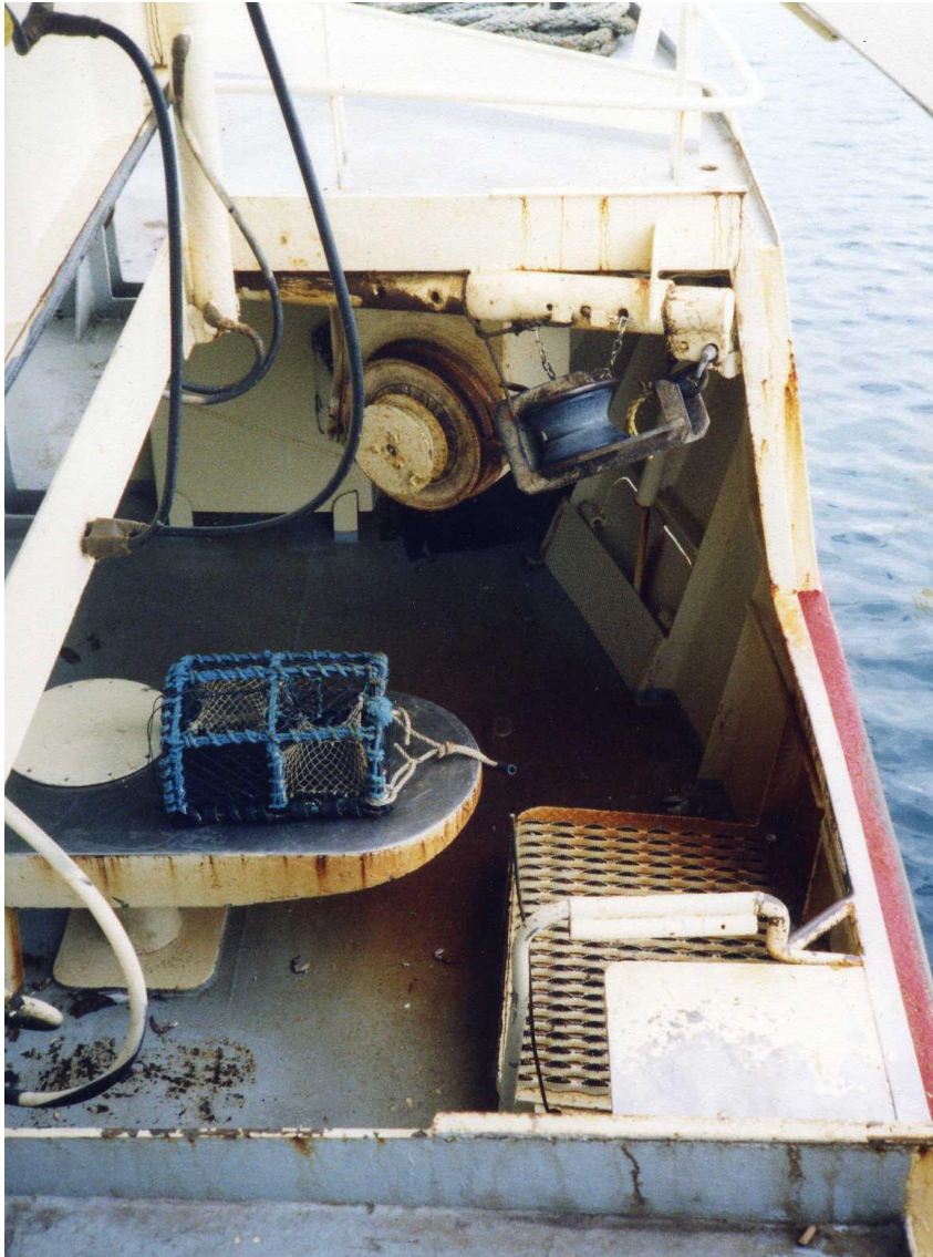
Line hauler with davit and open snatch block stored in the retracted position
